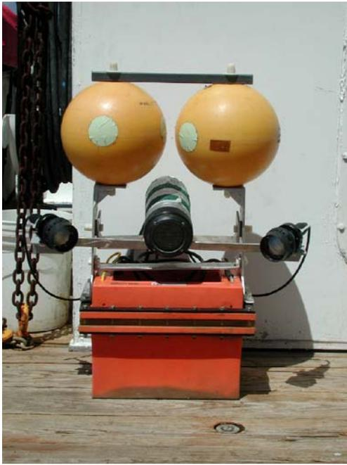
**Fig. 2** Time-lapse camera that was deployed at Bush Hill, displaying floats, lights, pressure-housing, and battery case. Spherical floats provide compensating buoyancy and a righting moment
